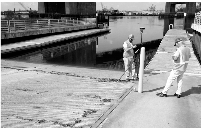
Forrest Ashley and Ed Ashworth verifying the high waterline marks. The debris line from high tide is visible.
